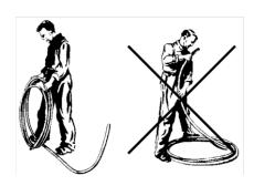
2. Metal hoses must be installed without interference in their natural position and in movement, do not allow the installation to reduce the value specified by the manufacturer minimum bending radius of the metal hose.
